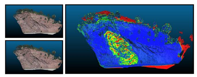
Figure 3.2 Colorado DOT rockslide change detection
