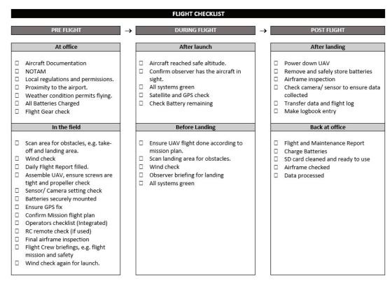
Figure 1: Example of a Flight Checklist\*
