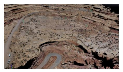
Figure 3.26 3D point cloud of Moki Dugway
